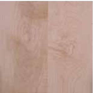
MAPLE , Hard A very strong hardwood with a closed, subdued grain and a uniform texture.
