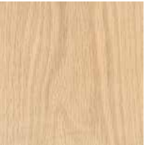
OAK , Red A hardwood chosen mainly for its prominent open grain pattern. Some color variation from reddish-tan to medium brown.
