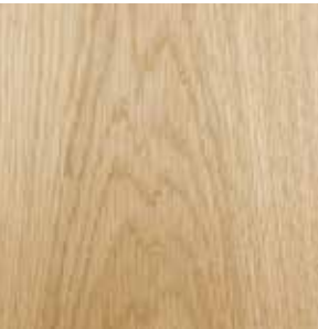
OAK , White A dense hardwood with a white to cream to light brown color, and longer grains than Red Oak.
