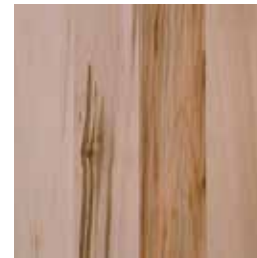
MAPLE , Wormy Selected to show mineral streaks and color variations caused by the ambrosia worm.
