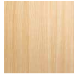
BEECH With exceptional color uniformity and texture, the lumber is steamed to a consistent tan color.
