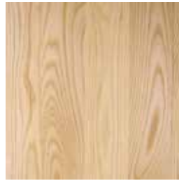
ASH , Northern White Valued for its strength, hardness, heavy weight, and elasticity, its use in baseball bats is famous.
